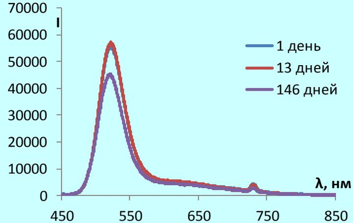
Fluorescence spectra in water, excitation with UV filtered by UFS-2
