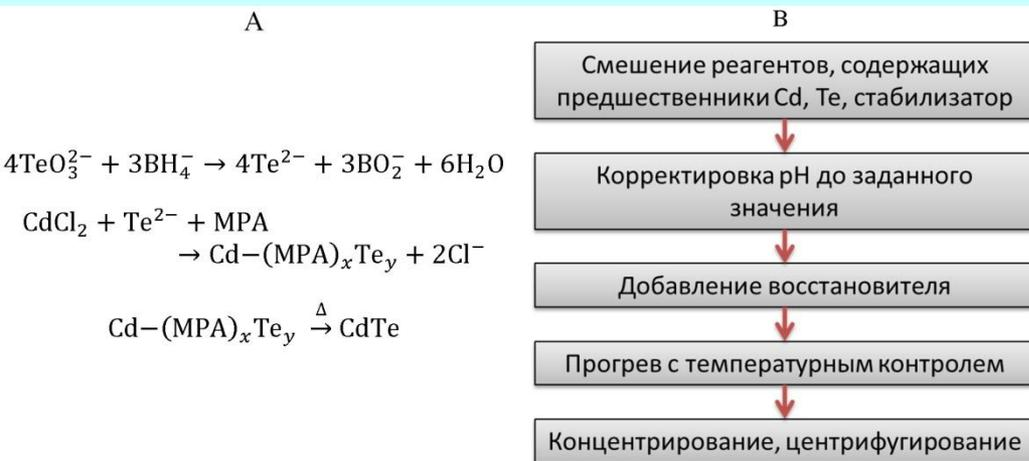
Fig. 1. A - Basic chemical reactions in the technology of obtaining CdTe QDs stabilized with 3-mercaptopropionic acid (MPA), B - Basic technological stages of the synthesis of CdTe QDs.
