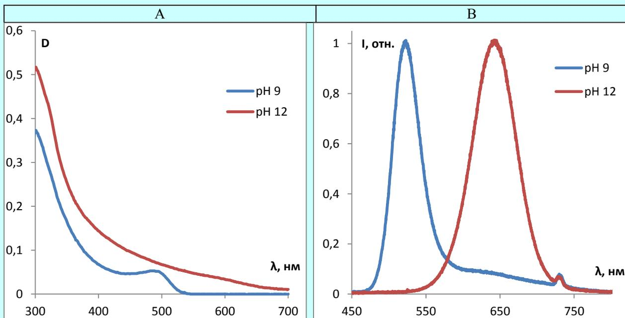
Fig. 3. Electronic spectra of CdTe QDs preparations (A) and their fluorescence spectra (B).
