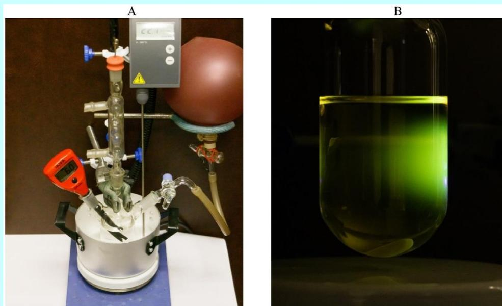
Fig. 2. A - General view of the installation for producing CdTe QDs stabilized with 3-mercaptopropionic acid, B - "Light beam in the dark kingdom" - fluorescence of the CdTe QDs reaction mix after reflux before the stage of separation  $\lambda_{\text{max fl}} 520 \text{ nm}$ .
